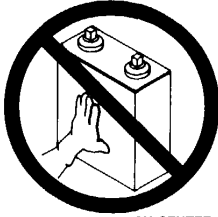
DO NOT PUSH ON CENTER TO POSITION BATTERY
